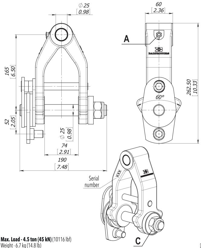
Pin locking nut (C) has to be tightened with a torque of 60-160 Nm (45-120 lb ft) dependent on desired brake power. Fill grease Statoil Uniway Li62 (or equivalent) through lubricating nipple (A), until it will appear to the external surfaces. Greasing must be repeated after every 8 working hours of the link.
